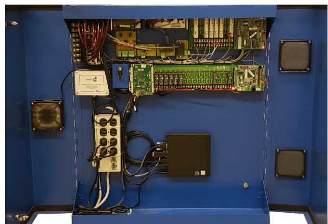
Electronics cabinet open with easy access to all components
