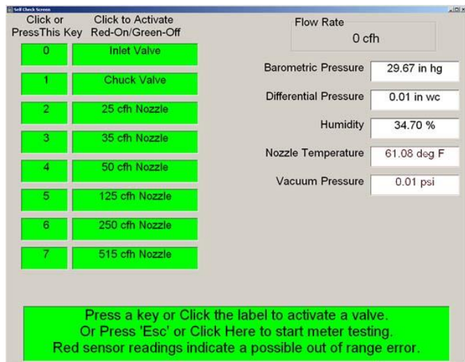
All valves can be operated and sensors monitored in real time allowing simple and straightforward troubleshooting.
